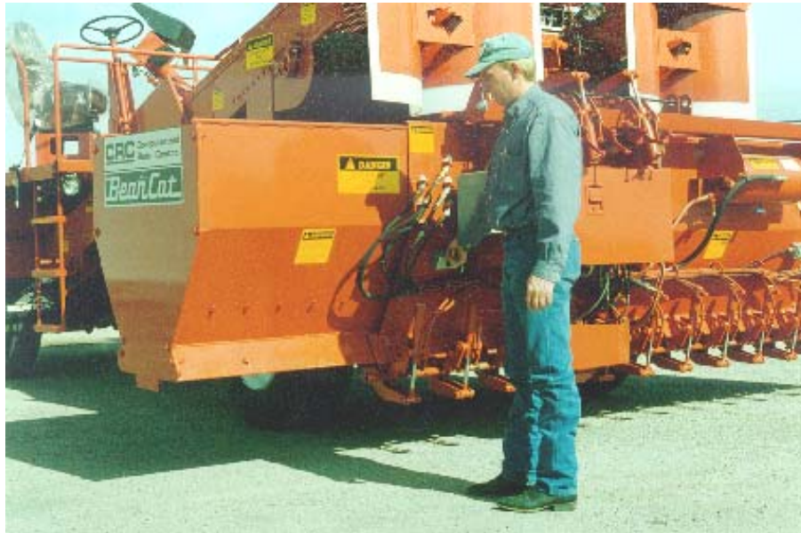
Figure 3-9. Expanding the Chip Box
