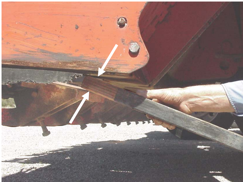
Figure 6-2. Checking Gate Opening
