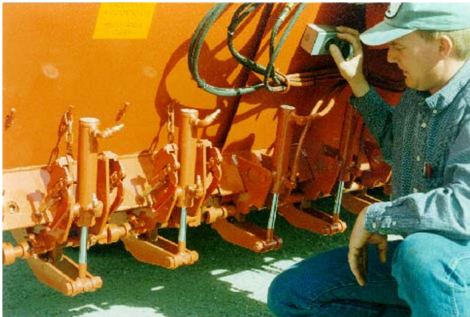
Figure 3-18. Closing the Chip Box Extension
