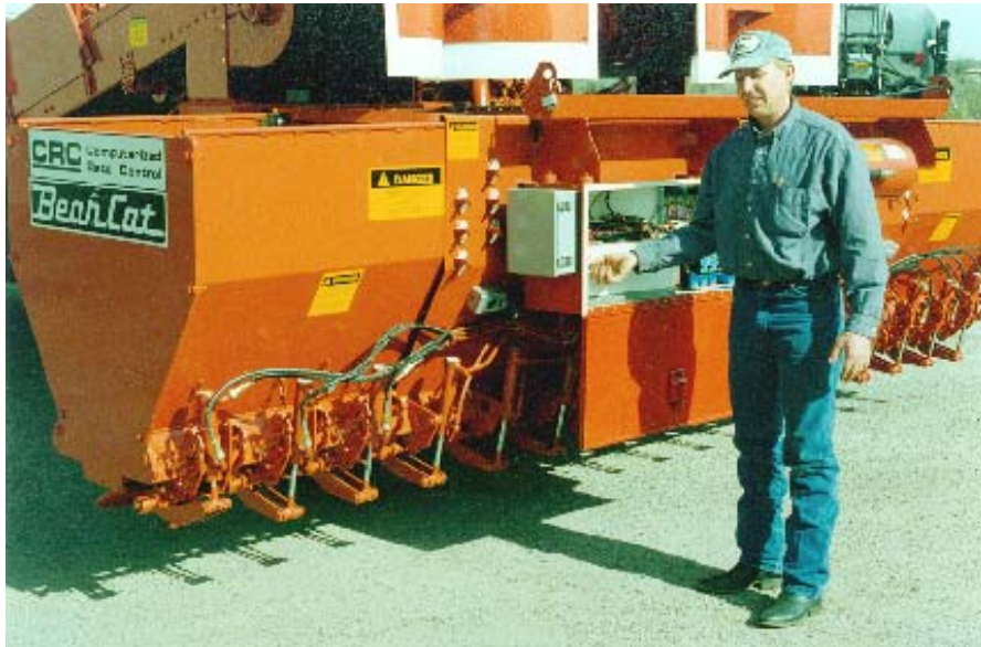
Figure 3-25. Testing the Gate Operation
