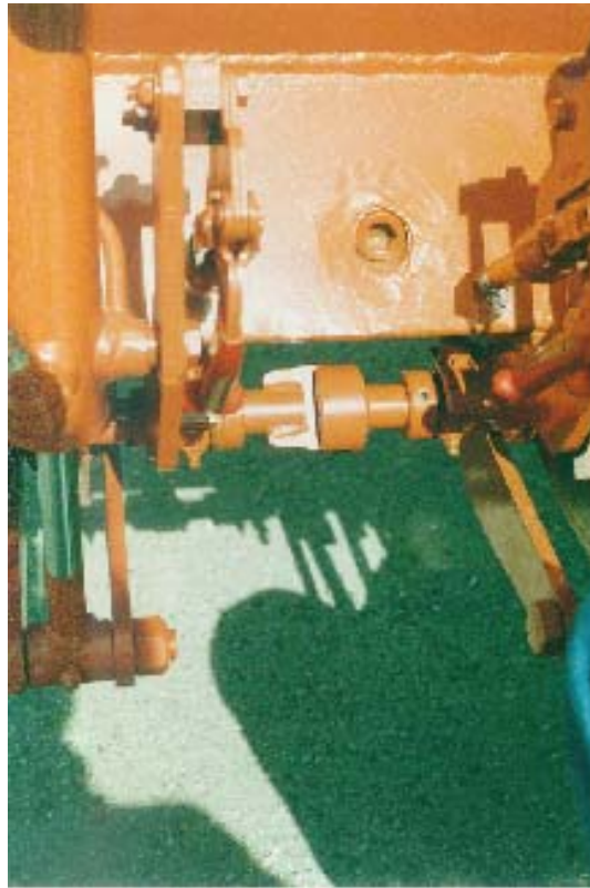
Figure 3-20. Proper Gate Cam Alignment
