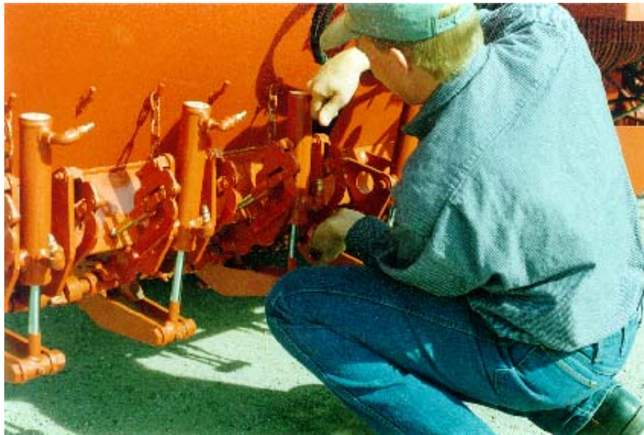
Figure 3-17. Adding the Inside Additional Gate
