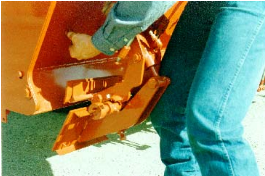
Figure 3-12. Hanging the Gate
