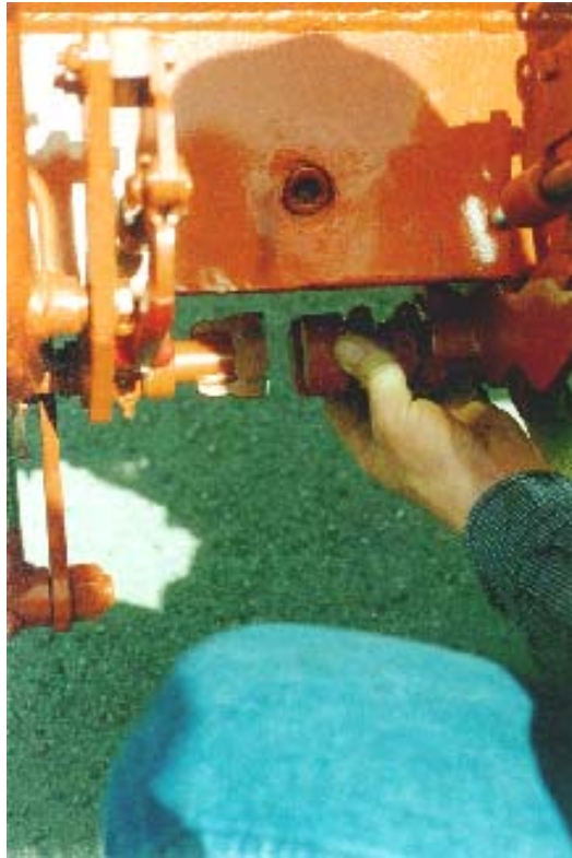
Figure 3-19. Aligning the Extension Gate Cams
