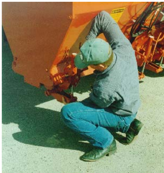
Figure 3-14. Adjusting the Gate
