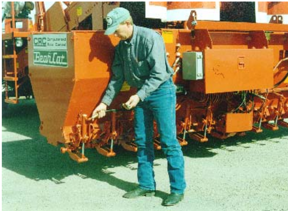
Figure 3-22. Attaching the Short Air Hose
