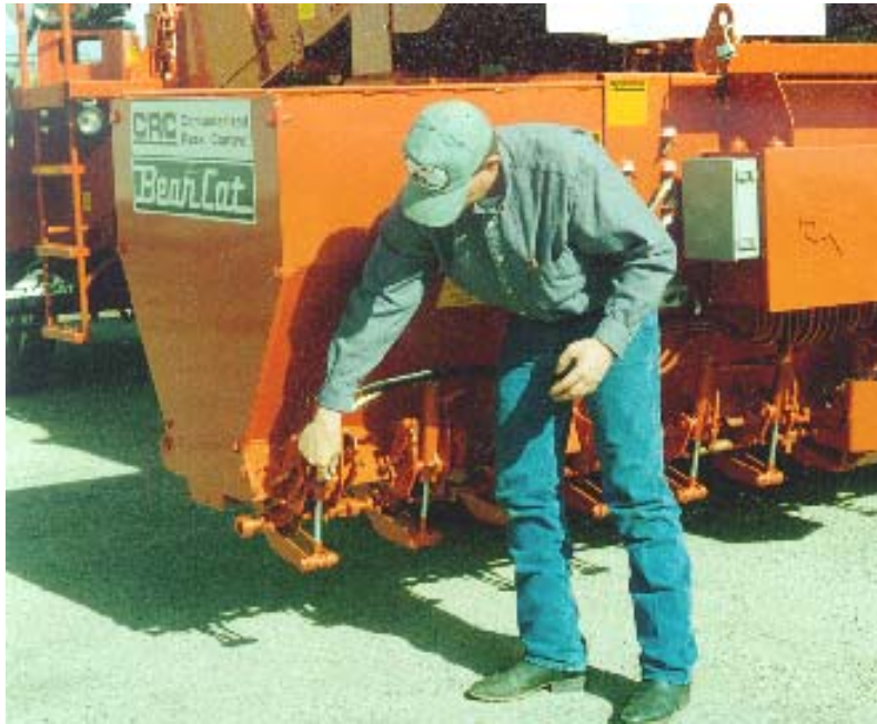
Figure 3-23. Attaching the Long Air Hose
