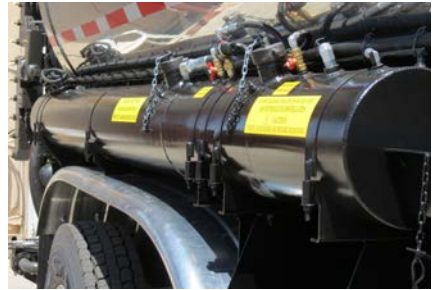
Flush and Washdown Tank
