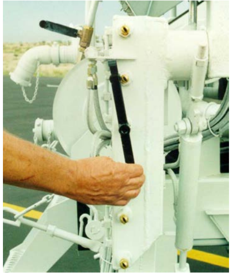
Alignment of Spray Nozzle
