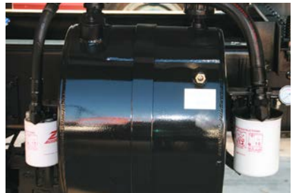
Hydraulic Reservoir and Filter
