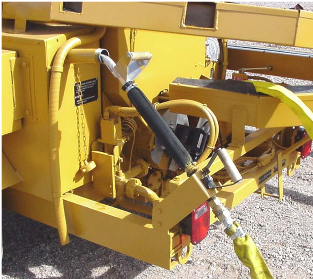
Figure 1-26. Application Wand in Return Tube and Bracket Assembly
