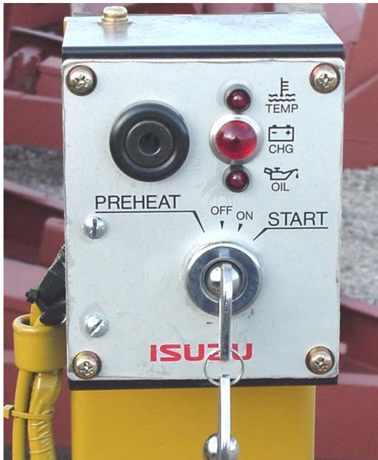
Figure 3-1. Engine Control Panel
