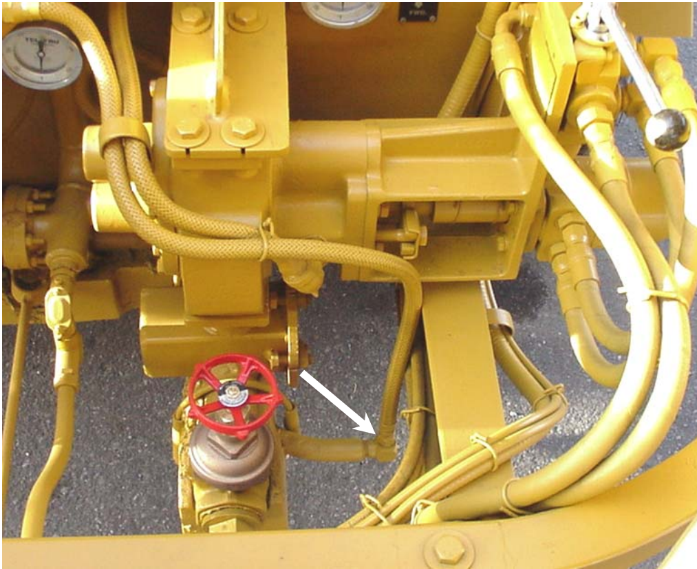
Figure 5-2. Bottom Flex Line Fitting
