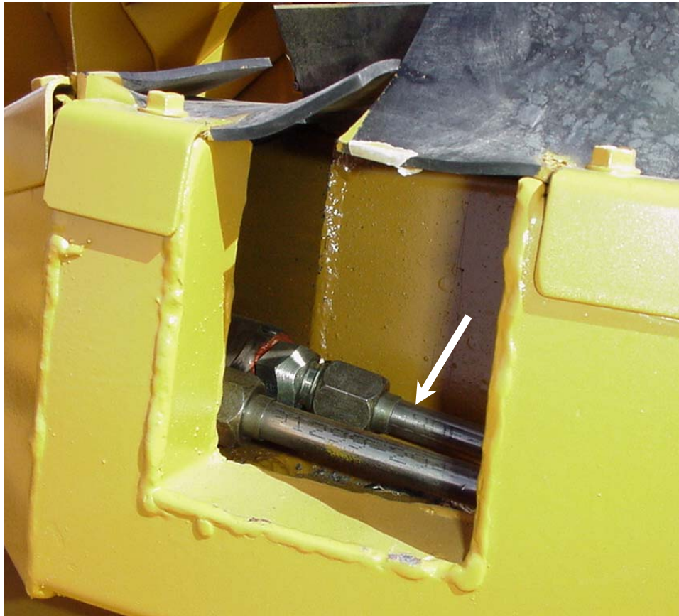
Figure 1-27. Heat Trace Lines
