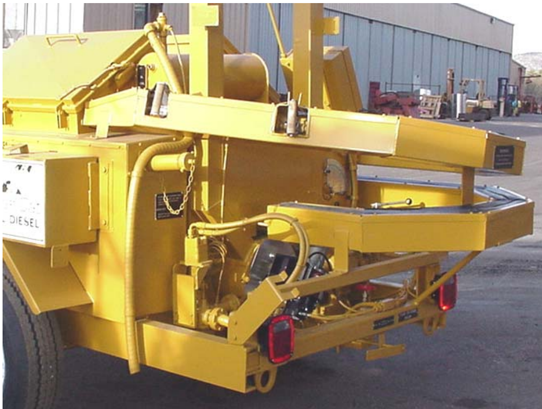
Figure 1-28. Application Wand In Hose Trough
