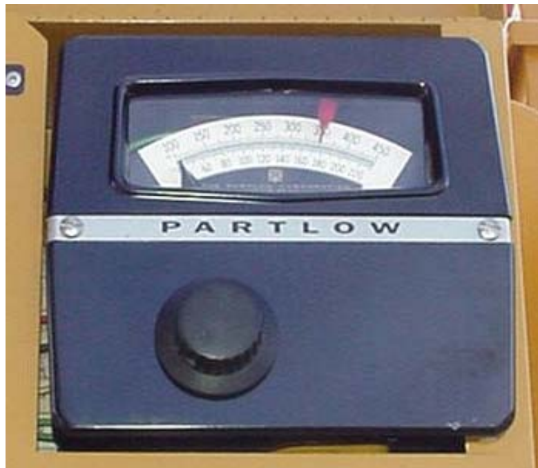
Figure 1-17. Partlow Sealant Temperature Control
