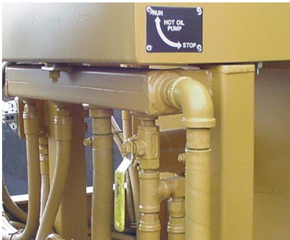
Figure 3-4. Hot-Oil Bypass Valve (STOP position)
