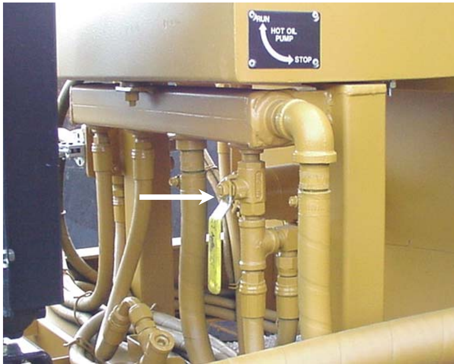
Figure 1-9. Hot-Oil Bypass Valve
