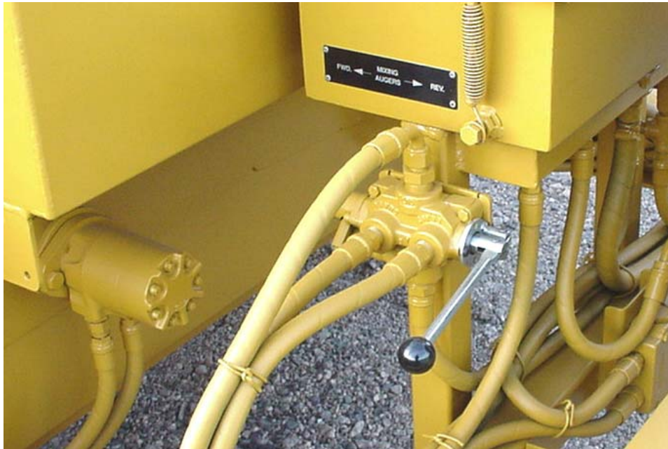
Figure 1-5. Directional Control Valve and Auger Motor
